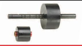
All new wide track 1.5" (38.1mm) feed roll and pinch roll using a high coefficient of friction urethane insuring your tape is always on the move. Provides quiet and accurate tape feeding. Creates less dust; less cleaning, adjustment and won't damage tape.
